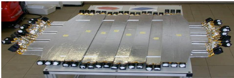
Figure 4.16: Picture of a pair of TOF planes.
