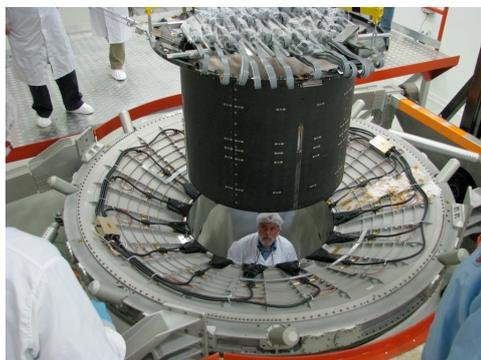
Figure 4.14: AMS-02 assembly trial: insertion of the Inner Tracker in the magnet vacuum case.
